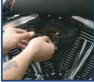
6. Install the secondary plate (9). Install the filter (8) and outer cover (II) at the same time using one I/4"-3/4" Cap screw (I) to hold the assembly in place. Install the remaining bolts and torque the bolts to 8 ft-lbs.
