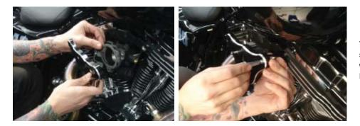
4. On Big Twin & Sportster models attach the backing plate(4) to the carburetor/throttle body using the supplied I/4"-20 x 5/8" socket head bolts(5) and tighten to 8 ft-lbs. On 2008-up FL touring models with electronic throttle locate the backing plate(4) to the throttle body using the supplied I/4"-20 x I-I/4" socket head screws. Do not tighten during this step.
