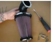
Slide the aluminum rear filter cover(14) off the filter onto the 90degree tube(12) to expose the hose clamp(15). Tip: Place masking tape around the 90degree tube(12) to protect the finish from damage! Loosen the hose clamp to free the filter element(16).
