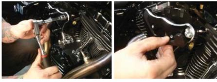
7. On Big Twin & Sportster models using the supplied  $1/4"-20 \times 3/4"$  socket head bolts(10) install the secondary plate(8), gasket(II), and complete filter assembly(9) and torque to 8 ft-lbs. On 2008-up FL models with electronic throttle install the secondary plate(8), gasket(II), and complete filter assembly(9) using the  $1/4"-20 \times 1-1/4"$  socket head screws and torque to 8 ft-lbs.
