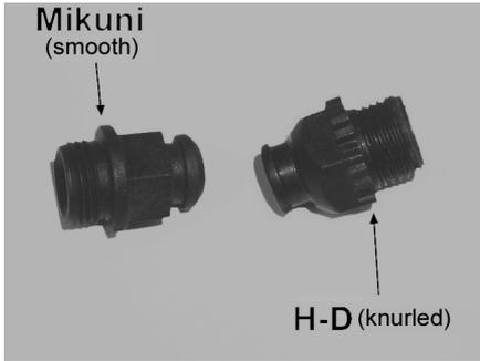
The Mikuni nut has a smaller hole where the cable fits and must not be used with the Harley choke cable.
