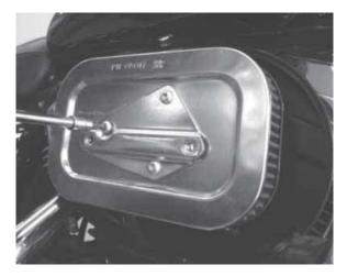
**1.3)** Remove the stock breather bolts and throttle body bolts. On some models there will be vent lines being fed to the air filter assembly, remove these and re-route them to beneath the engine. Remove the stock breather box.
