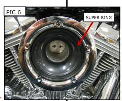
STEP 13 Double check the tightness of all related fasteners, check for hose clearance and check throttle for correct operation, making sure it returns properly, before starting bike.
