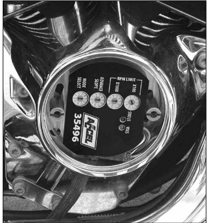
Figure 3A - Finished Big-Twin® Installation
