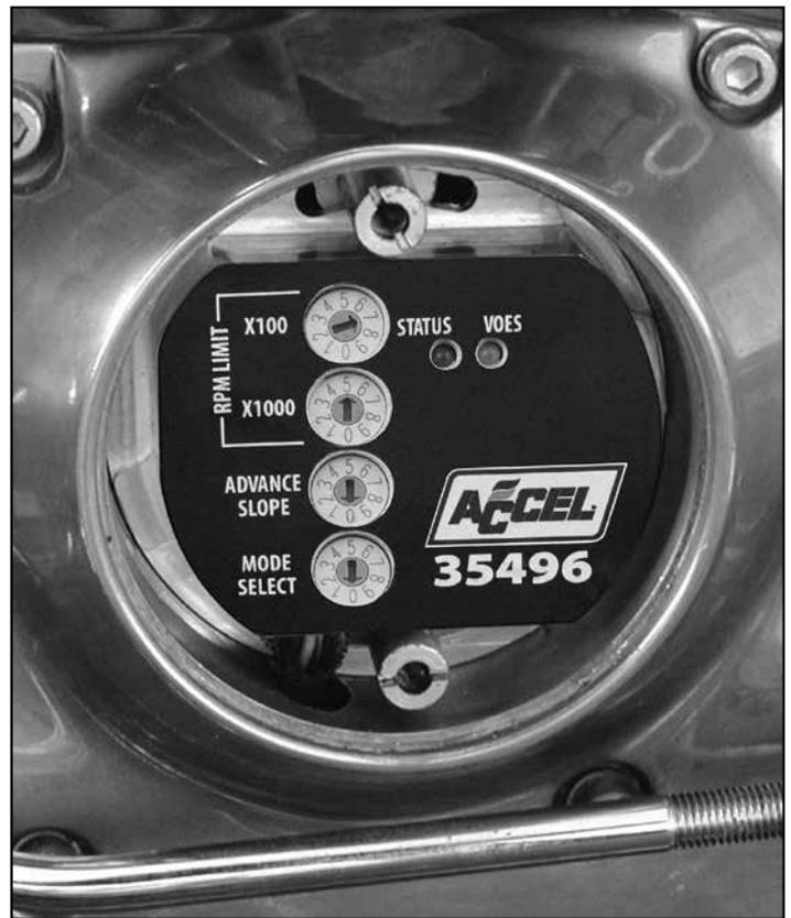
Figure 3B - Finished Sportster® Installation
