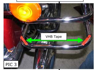
Note the curve of the mounting plate and which way it is facing. Notch towards the front.
