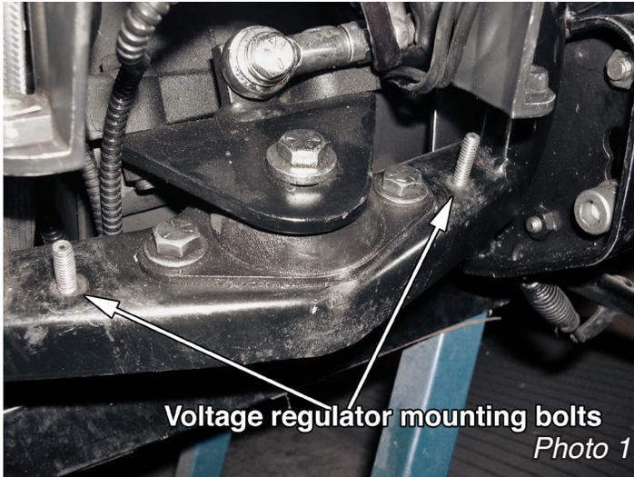
23. Using the 1/4-20x3/4" button head bolts included in the kit, install the voltage regulator riser brackets to the bottom of the voltage regulator mounting feet. The "open" side of the riser brackets should orient to face toward the horn side of the motorcycle when installed (to allow clearance for the oil hose).
