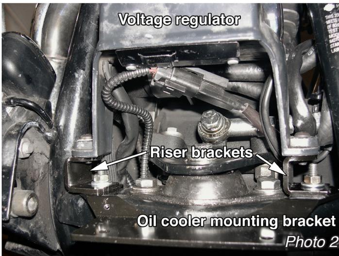
24. Install the oil cooler mounting bracket over the voltage regulator mounting bolts, taking care not to pinch any electrical wires.
