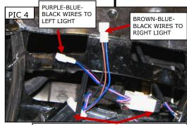
WIRING ADAPTER CONNECTED TO MAIN HARNESS
