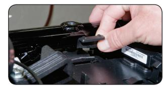
3. Cut and remove the left ECU hold down to allow the ECU to slide over.
