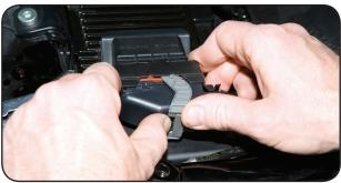
Remove seat, exposing factory computer (ECU). disconnect factory wiring by pressing lock and pushing lever back.
