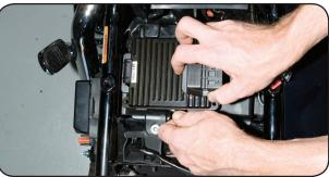
Remove ECU by pushing tab and sliding the ECU to the right as you lift.
