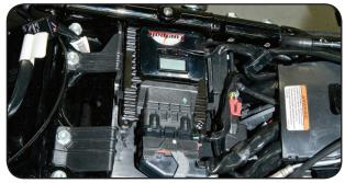
Attach Fuelpak to the top of the ECU by using the supplied Velcro.
