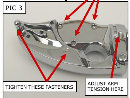
**WARNING** CHECK TO MAKE SURE THAT THERE IS PROPER GROUND CLEARANCE WITH AND WITHOUT THE FOLDING ARM EXTENDED WHEN CORNERING. LOSS OF CONTROL OF THE MOTORCYCLE AND SERIOUS INJURY MAY OCCUR IF THE FLAMIN' SWITCHBLADE PEG IS NOT POSITIONED PROPERLY. REPOSITION THE FLAMIN' SWITCHBLADE PEG IF NECESSARY SO THAT THERE IS ADEQUATE CORNERING CLEARANCE.
