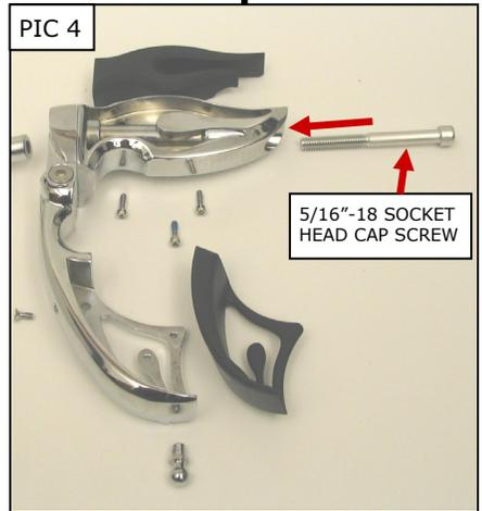
**ADJUST DETENT SPRING TENSION**
