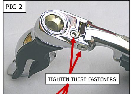
**WARNING** FOOTPEGS MUST BE INSTALLED SO THEY WILL FOLD UPWARD AND REARWARD IF HIT BY ANY OBJECT. FAILURE TO ADJUST THE FOOTPEGS TO OPERATE IN THIS MANNER COULD RESULT IN SERIOUS INJURY OR DEATH.
