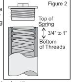
your fork caps have adjustable pre-load settings or are recessed below the edge of the fork tube (circlip type), then they are usually much longer than the ¾" to 1" caps and must be measured accordingly.
