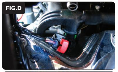
6 Locate the stock wiring harness at the rear injector (Fig. D). Remove the RED clip and unplug the injector connector.
