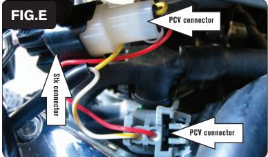
7 Plug the YELLOW colored wires from the PCV in-line of the stock wiring harness and fuel injector (Fig. E)
