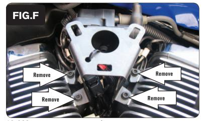
Remove the 4 bolts that hold the Ignition coil bracket to the engine (Fig. F).
