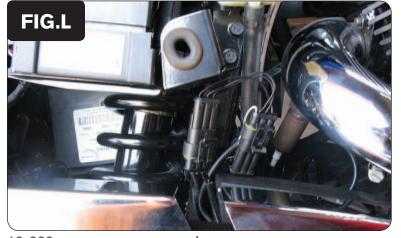
17 Plug the PCV harness in-line of the stock wiring harness and crank pickup coil connector (Fig. L).
