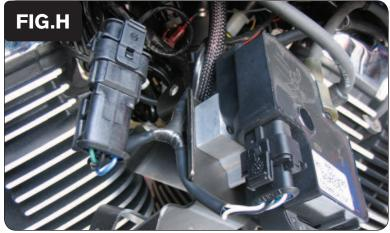
11 Plug the PCV wiring harness in-line of the stock wiring harness and Ignition coil (Fig. H).
