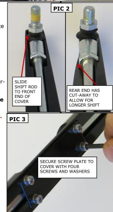
REMOVE THE FRONT END FIRST, THEN THE REAR END
