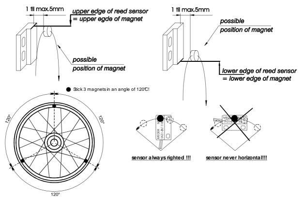
Install the sensor and the magnets according to the sketch. The mentioned dimensions refer to the reed sensor of  $\textit{MMB}^{\text{®}}$ .
