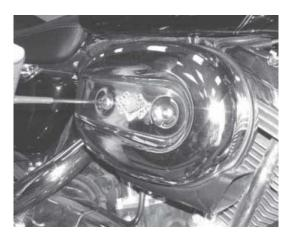
**1.2)** Remove the three T25 Torx screws that secure the stock filter. Remove the gasket from the stock filter and set aside for later use.
