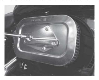
1.3) Remove the stock breather bolts and throttle body bolts. On some models there will be vent lines being fed to the air filter assembly, remove these and re-route them to beneath the engine. Remove the stock breather box.
