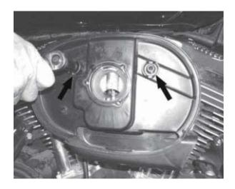
**1.4)** Remove throttle body support (fuel injected models) by removing the bolt in the center.
