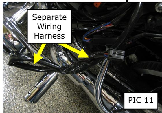
**ATTENTION!** Secure all wiring away from any moving parts, pinch points or extreme heat. Kuryakyn WILL NOT warranty any electrical component that fails due to pinched, crimped, broken, abraded, melted or frayed wires.
