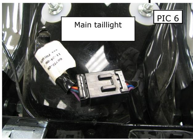
**Note:** For '93-'96 models, it will be necessary to hardwire the lights, skip to STEP 26 under the wiring procedure for '93-'96 section.
