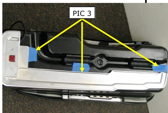
**STEP 9** Using the back of your fingernail, rub the backing of the adhesive pads to activate the adhesive.
